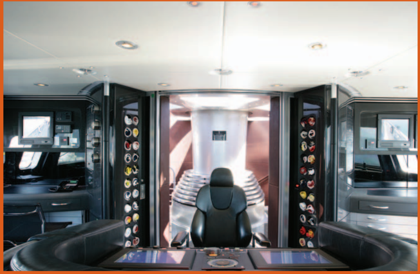
Above and below: The DynaRig and sails are fully computer controlled from an out-of-this world high technology helm display. Stresses in the rig sensed by fibre optic monitors are constantly displayed and all sail handling is fully automated.
