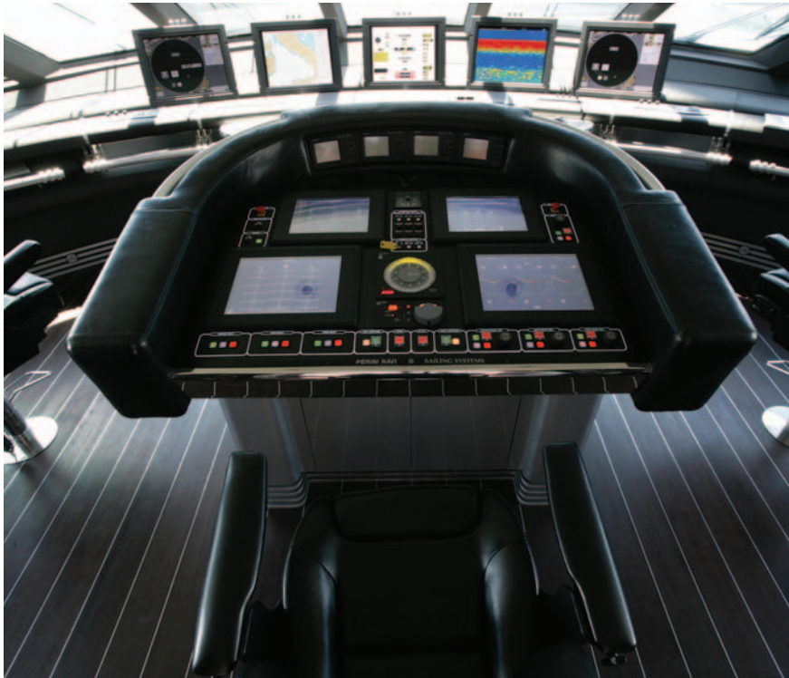
Above and below: The DynaRig and sails are fully computer controlled from an out-of-this world high technology helm display. Stresses in the rig sensed by fibre optic monitors are constantly displayed and all sail handling is fully automated.
